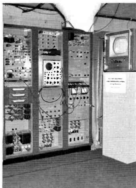
TEST EQUIPMENT FOR VIDEO DISTRIBUTION SYSTEMS . . . The use of RCA Test Equipment, Color and Monochrome was demonstrated in this area. Special attention was devoted to the use of RCA color units in checking existing monochrome systems so they may be adapted for future color use.
