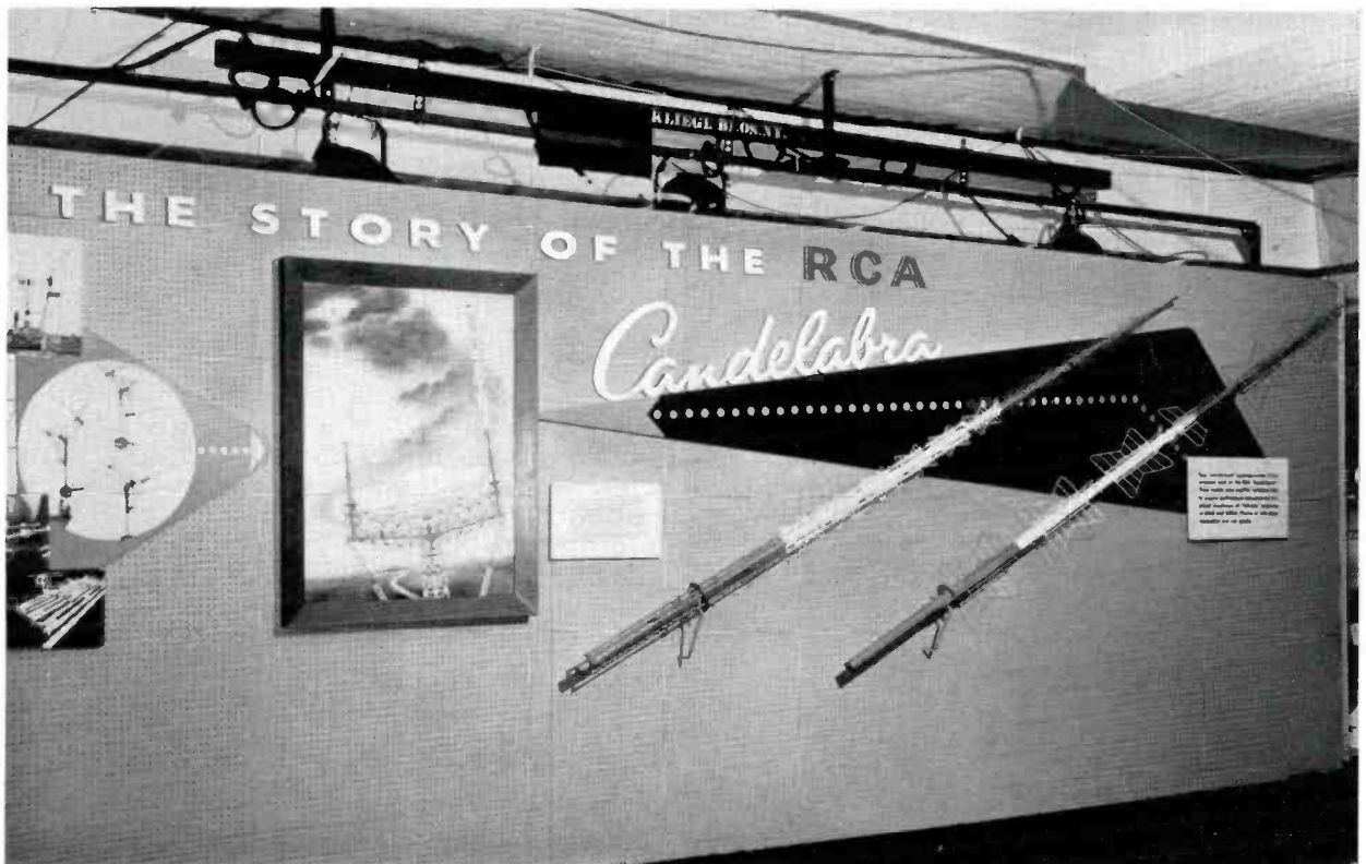
THE STORY OF THE RCA CANDELABRA . . . On the back wall of the color studio, the development story of the KRLD/WFAA antenna project is shown. Here miniature scale models used for engineering tests are displayed (right). Looking left is an artist's conception of the final installation and a photo mural showing the scale models being tested at the RCA Plant.
