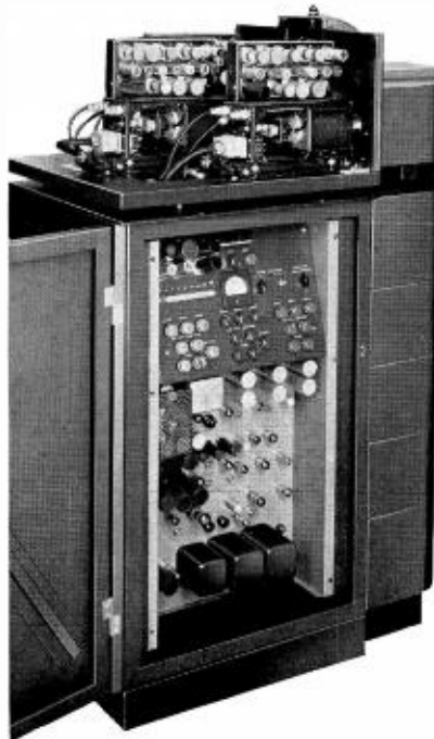
FIG. 10. Pedestal assembly supports optical system and houses camera auxiliary chassis.
