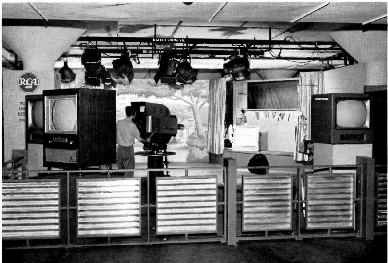
OVERALL VIEW OF LIVE COLOR STUDIO . . . The color studio occupied 900 square feet. Two separate sets, a puppet stage and a park scene occupied this area. Studio pictures were seen on two 21 inch RCA Color TV receivers and on two 21 inch black-and-white utility monitors. The RCA TK-41 Live Color Camera operated throughout the exhibit hours.
