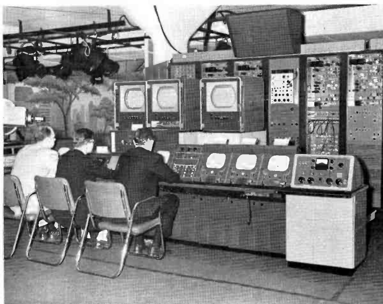
TELEVISION CONTROL CENTER . . . Control and rack equipments for all operating displays in the exhibit were located in this area. Color monitors (l. to r.) showed pictures from live color camera, 3-V color film camera, and color effects equipment. New masking amplifier for 3-V equipment is shown in front of the center monitor. Remote control panel for TP-15 Multiplexer is mounted in remote control housing (center).
