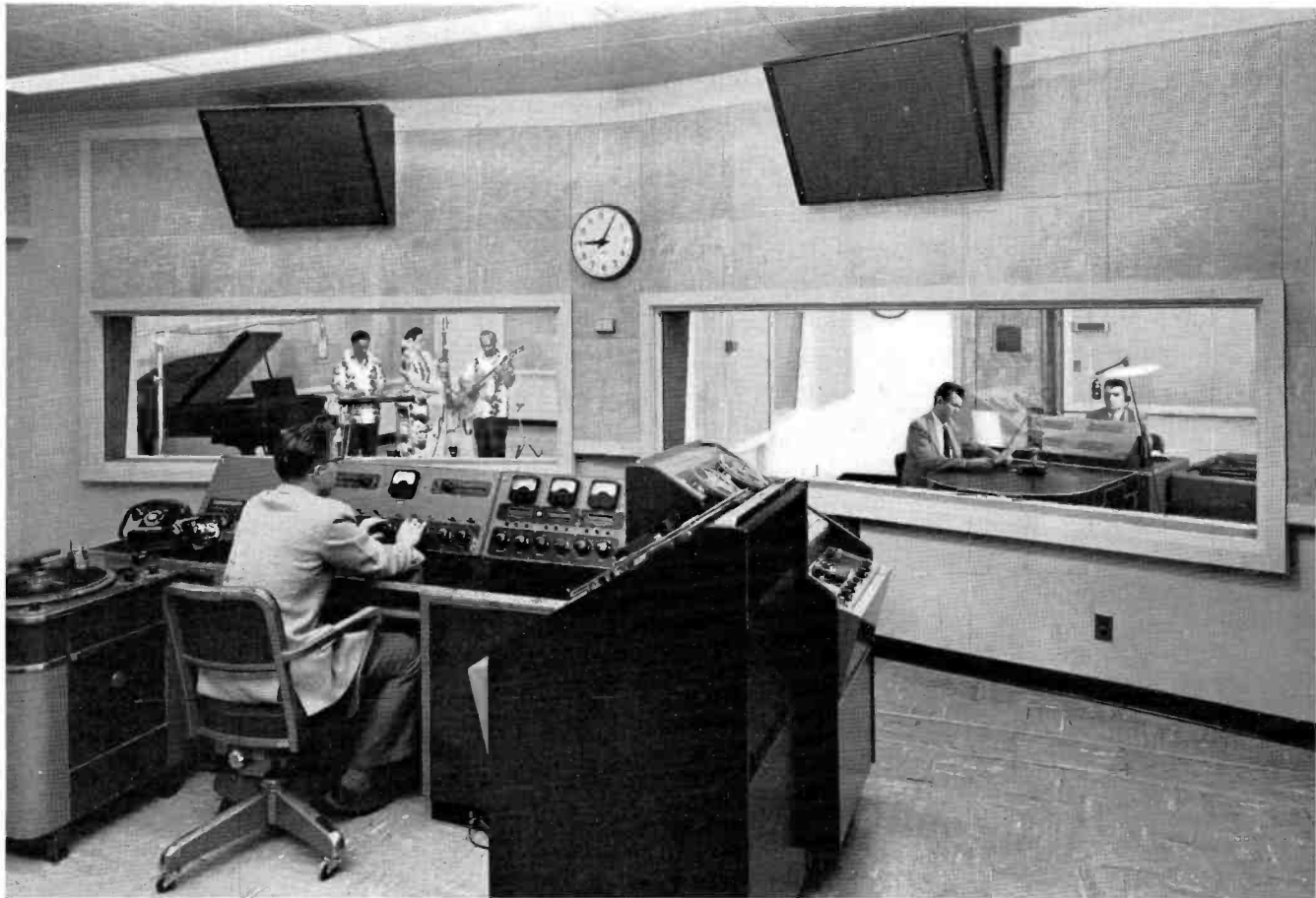
FIG. 14. AM Master Control Room in new WHIO Studio Building. The three AM studios are grouped about this control room so that there is direct visual communication between all three and the control room. An RCA BC-2B Console and RCA BCS-11A Switcher provide flexible facilities with a high degree of operating efficiency.
