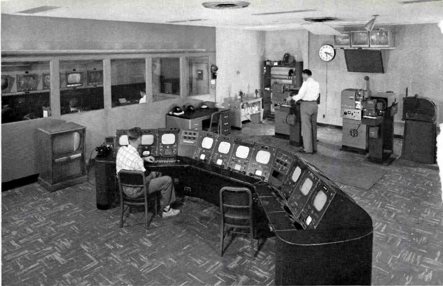
FIG. 9. WHIO's TV Master Control Room contains not only master switching equipment but also all camera controls and film projection equipment. Studio 2 camera control units are at left of main console; Studio 1 camera controls are at right; film camera controls, preview and line monitors are in the center.
