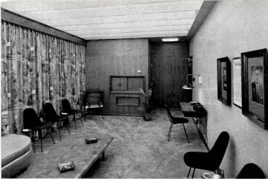
FIG. 16. This spacious and well-appointed conference room adjoins the manager's office in the new WHIO Building. The lighting system is unusual. Two 6-foot slimline tubes have been installed end-to-end and are supported by special steel channels which extend from wall to wall at 2-foot intervals. The channels also support V-shaped, perforated metal acoustic baffles. By mounting the tubes 18 inches below the reflective ceiling and operating them through remote ballasts, which are easily accessible on the opposite face of the wall shown here on the right, the engineers provided ideal lighting and eliminated any possibility of operating noise.
