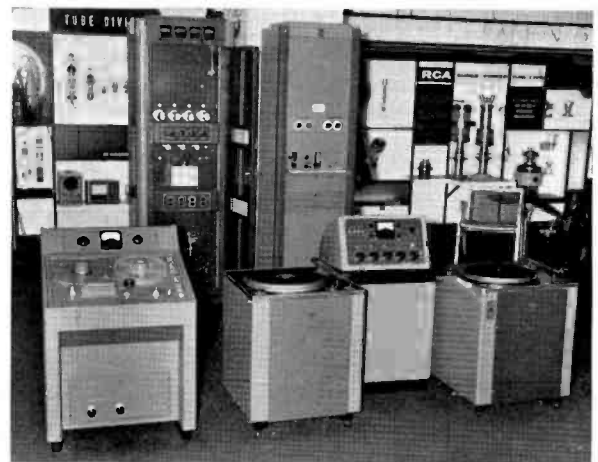
RCA AUDIO EQUIPMENT FOR AM/FM AND TV STATIONS . . . In the foreground (l. to r.) is an RCA console mounted tape recorder and two new BQ-2A Turntables flanking a BC-4A Audio Central. Cabinet racks house (left) a 250 watt AM Transmitter, and (right) a new line of printed circuit audio amplifiers.
